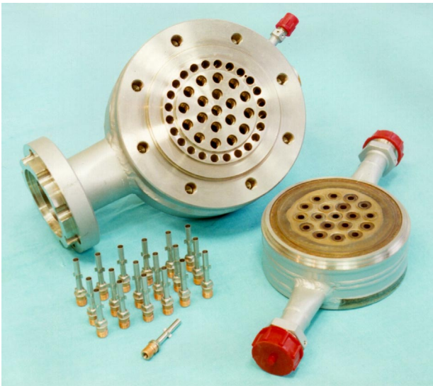
Figure 16: Subscale injection head parts
