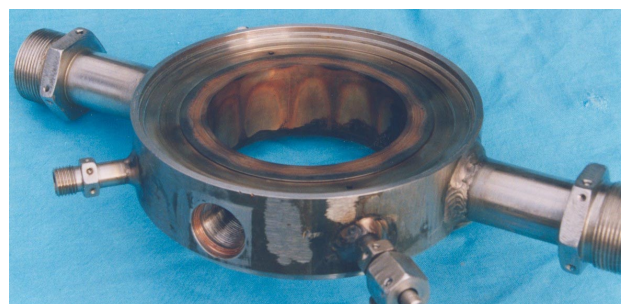
Figure 19: Chamber wall section after 12 tests showing discoloration due to heat load from injection elements
