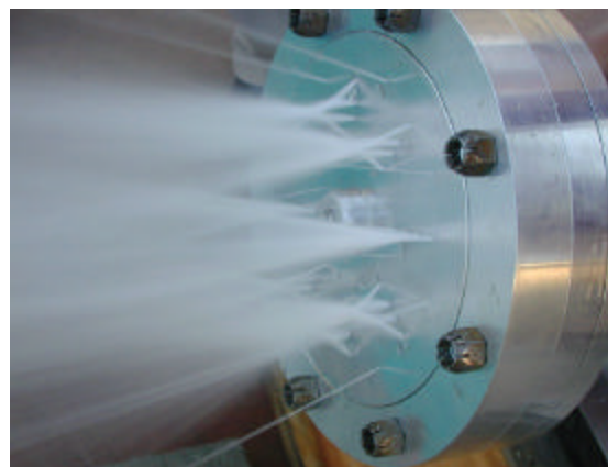
Fig. 13. Water flow test of the injector
