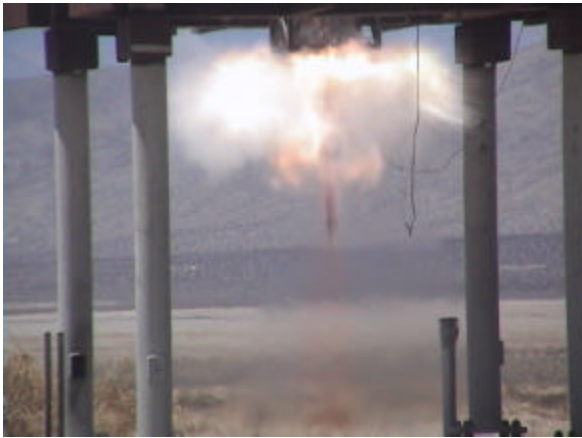
Fig. 16. Explosion in injector right after spike failure
