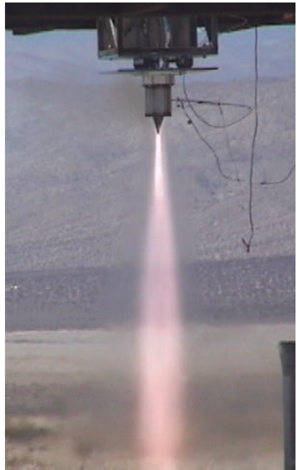
Fig. 15. Aerospike engine 200 ms after ignition
