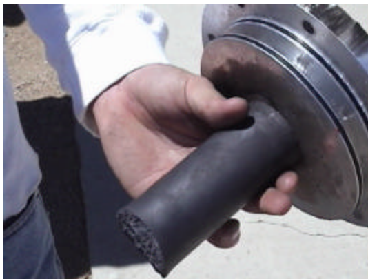
Fig. 17. Main injector plate and failed center rod
