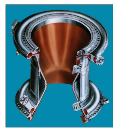
Geometry NARloy-Z liner + EDCu barrier + EDNi closeout + Inconel 718 structural Jacket + JBK-75 Cast Manifolds Number of slots 430 Injector end diameter (in) 17.74 Throat area (in<sup>2</sup>) 93.02 Injector end-to-throat length (in)
